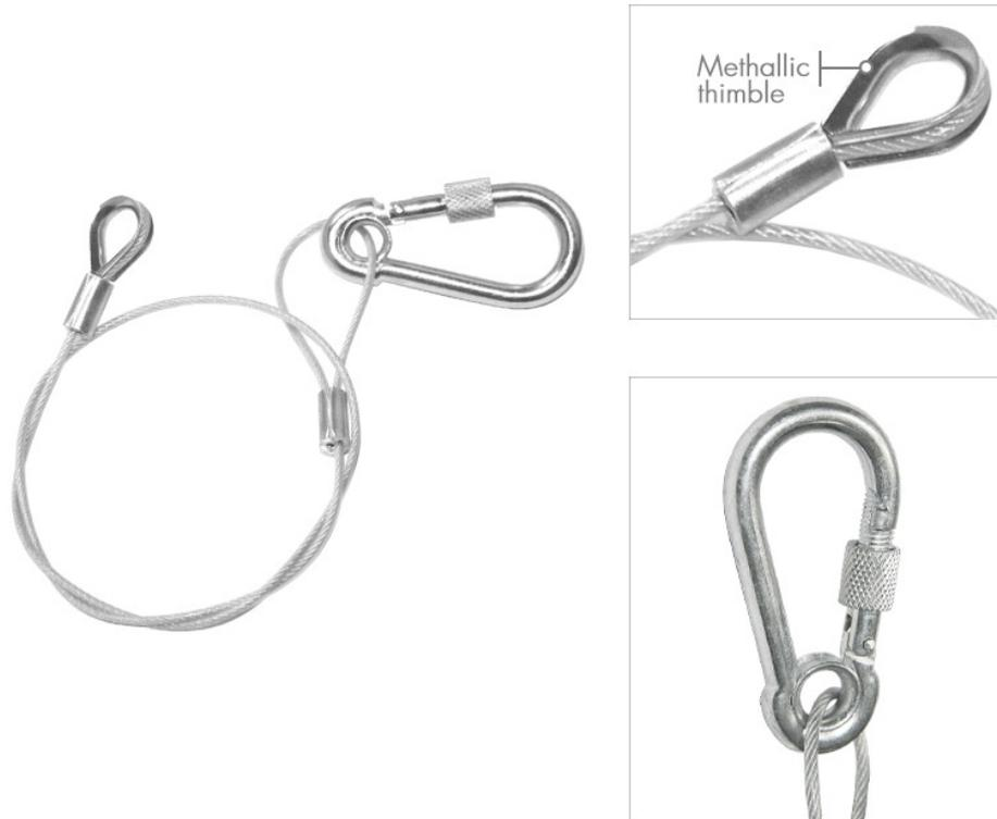
Stainless steel sling covered with transparent polythene (to not mark) with a maximum working load of 60 kg. It is provided with a carbine hook with a threaded locking sleeve (screw-lock). The screw lock prevents accidental or unwanted opening. The nut has a rough surface for a better grip when tightening it. Our safety bond has reinforced loop clamps at either end to guarantee maximum durability and comes with thimble eye to create the perfect reinforced eye loop.
